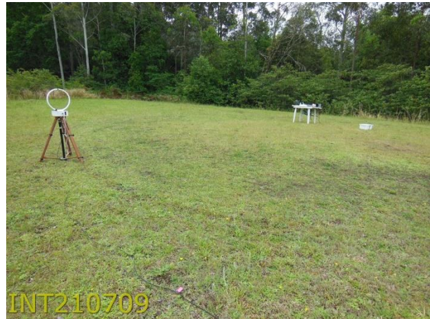
INT210709 Radiated <30 MHz No Ground Plane
