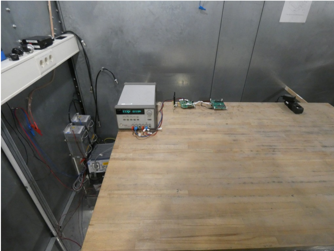
Photo 1: Test setup for conducted measurements below 30 MHz
