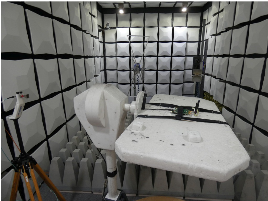
Photo 4: Test setup for radiated measurements above 26 GHz
