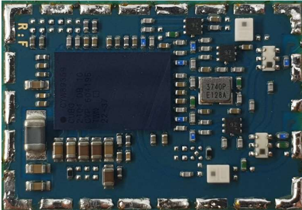
Figure 1: JODY-W164-03A internal photo
