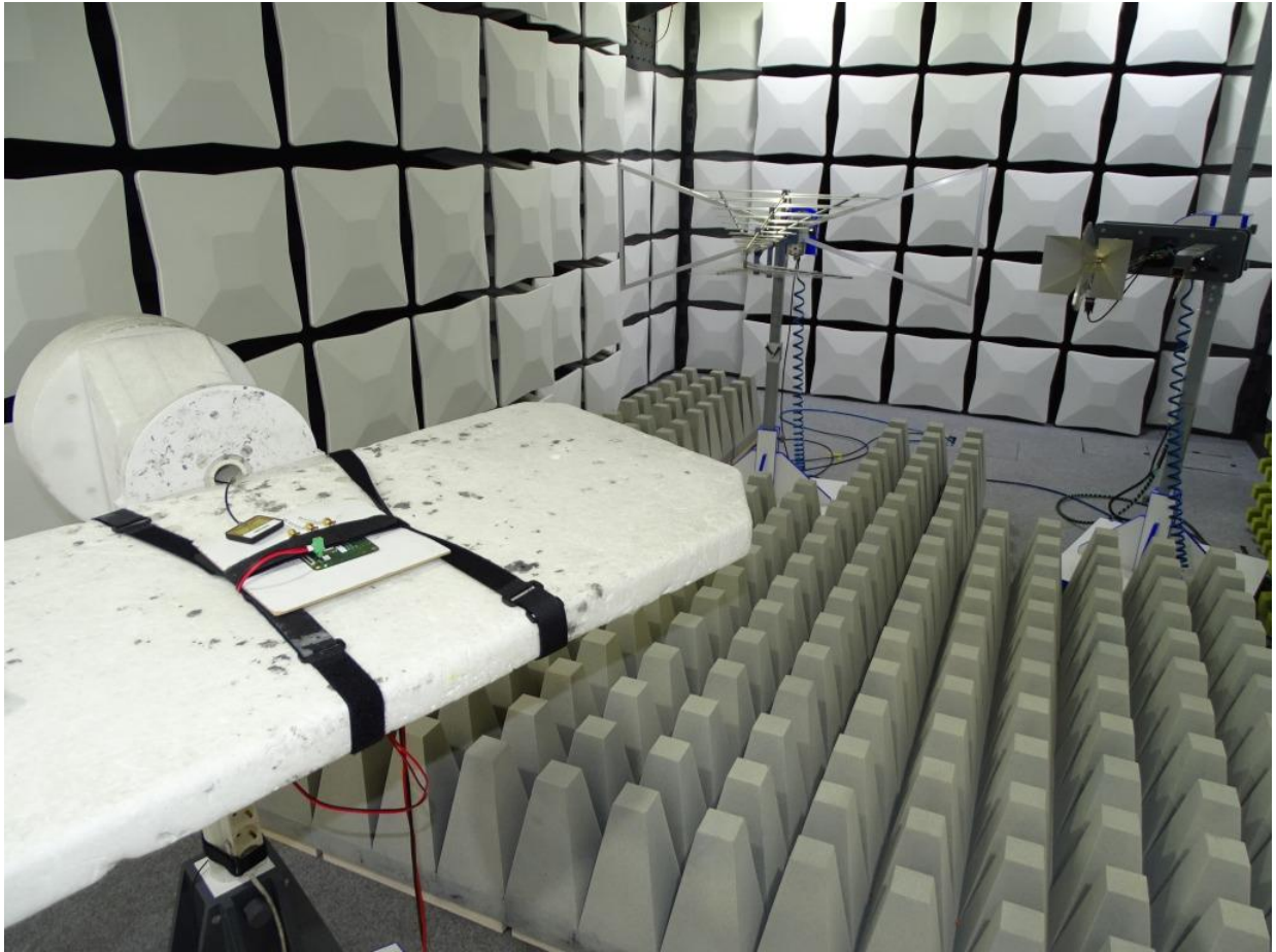
Photo 2: Test setup for radiated measurements above 1 GHz
