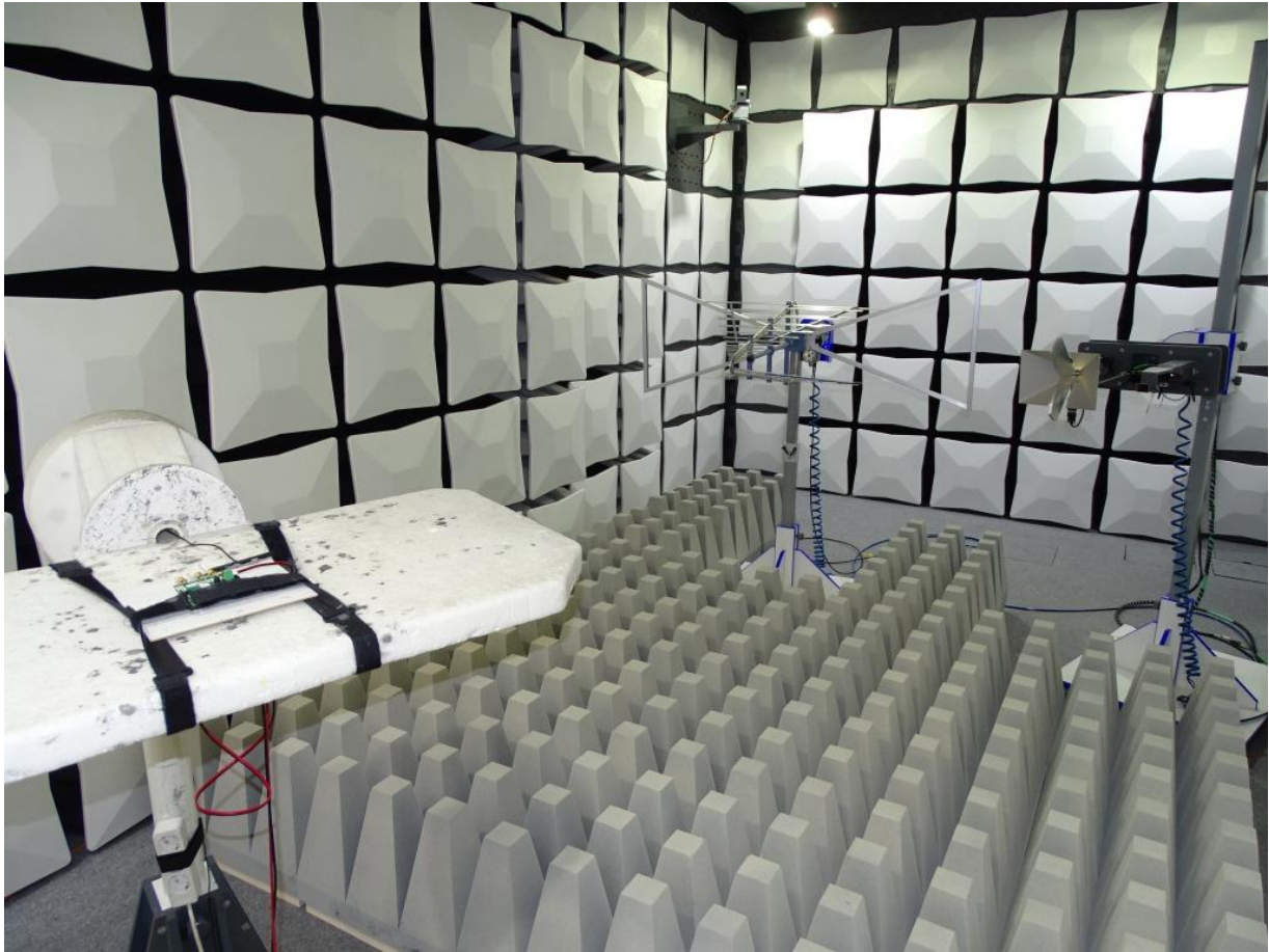
Photo 1: Test setup for radiated measurements above 1 GHz
