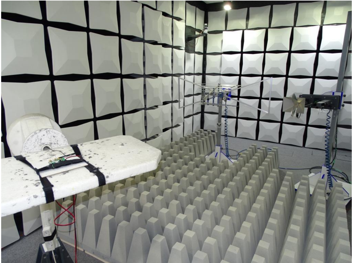
Photo 3: Test setup for radiated measurements above 1 GHz
