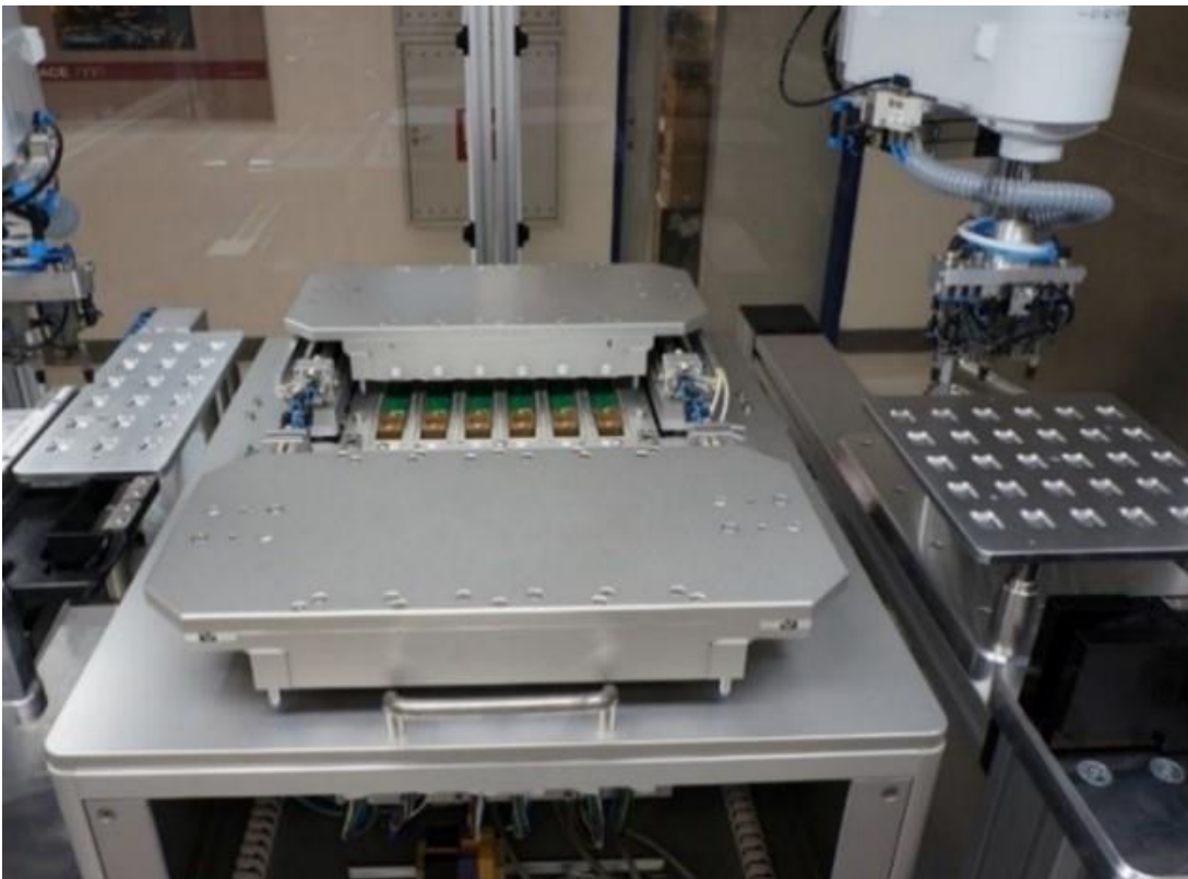
Figure 21: Automatic test equipment for module test
