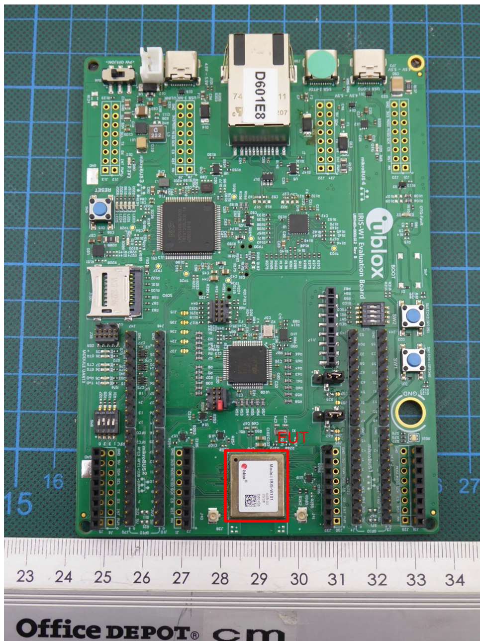
IRIS-W101-00B on evaluation board – top view
