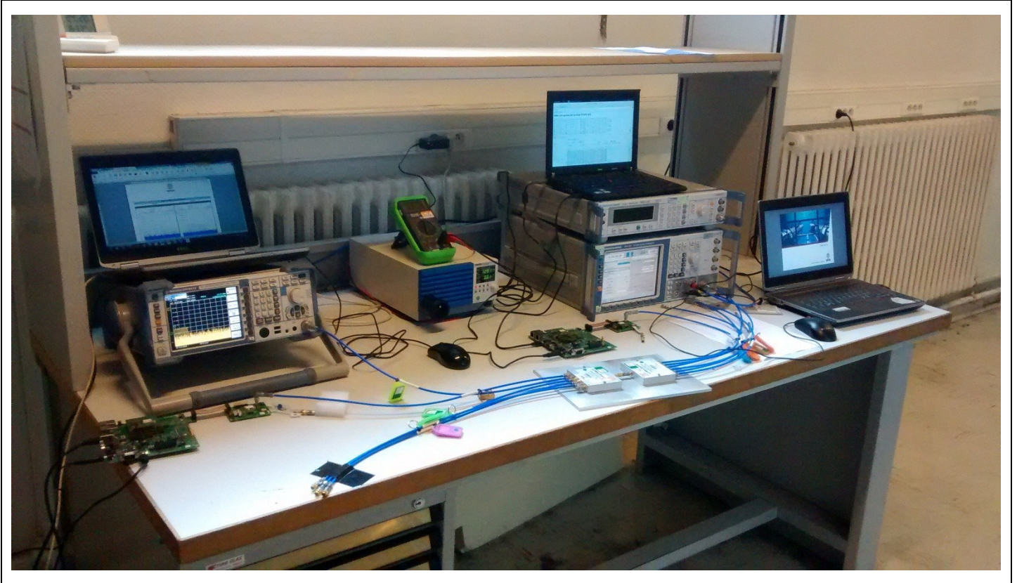
Photograph for DFS Detection Thresholds Determination, Reference Noise Level, Channel Loading
