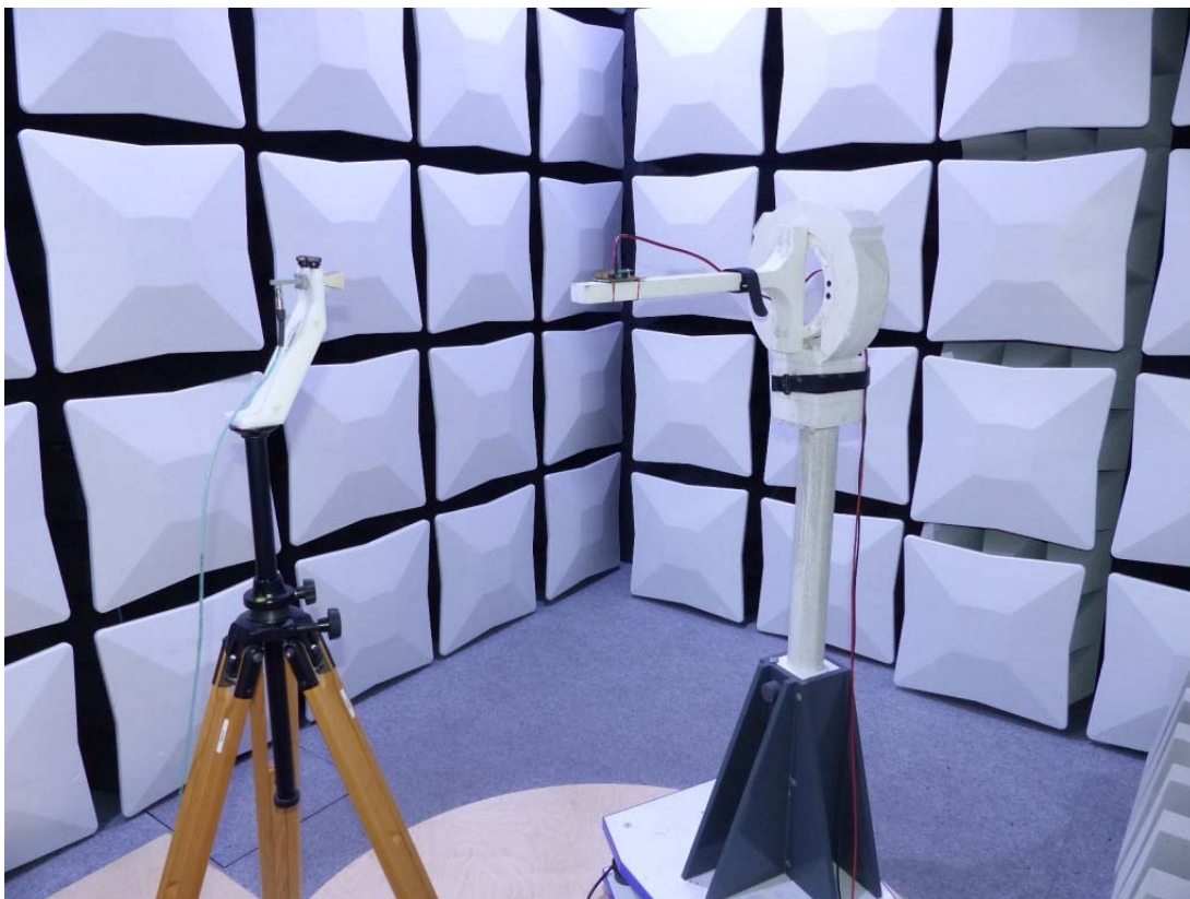
Photo 6: Test setup for radiated measurements (above 26 GHz)
