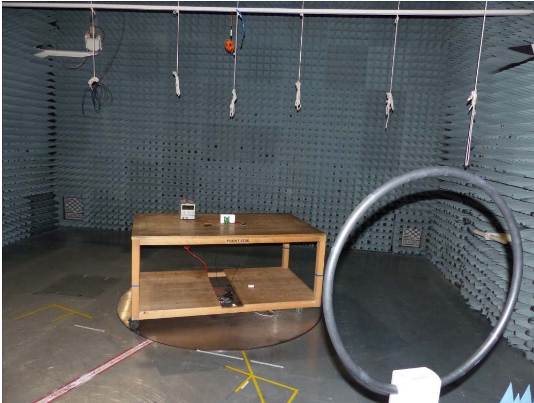
Photo 3: Test setup for radiated measurements (below 30 MHz)
