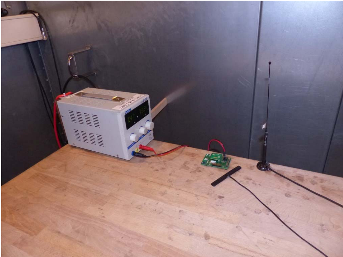
Photo 1: Test setup for conducted measurements at AC Port of lab power supply
