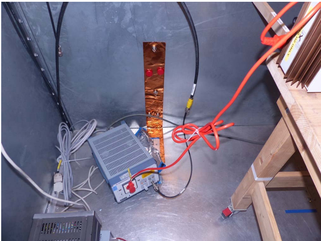
Photo 2: Test setup for conducted measurements (AC power line connected to LISN)
