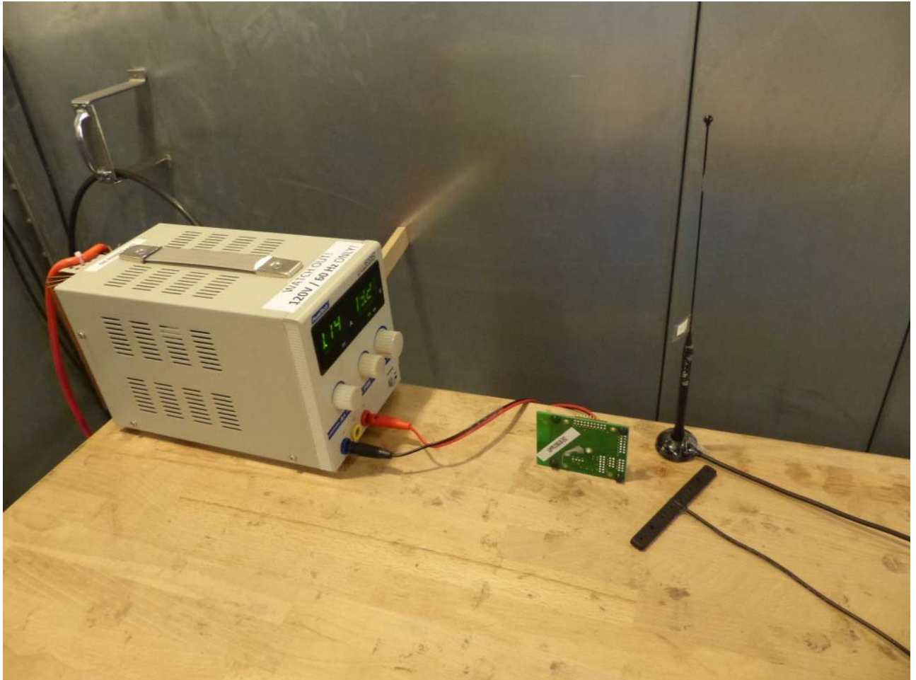
Photo 3: Test setup for conducted measurements (AC Port (power line), EUT supplied by AC/DC adapter, intentional radiator §15, ANSI C63.10 + KDB 174176 D01. EUT equipped with a real antenna.
