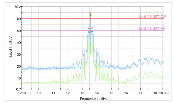
Note: Measured levels above the limit are from modulated carrier signal.
