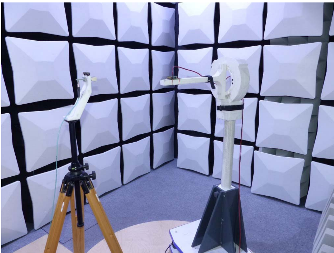
Photo 8: Test setup for radiated measurements (above 26 GHz)
