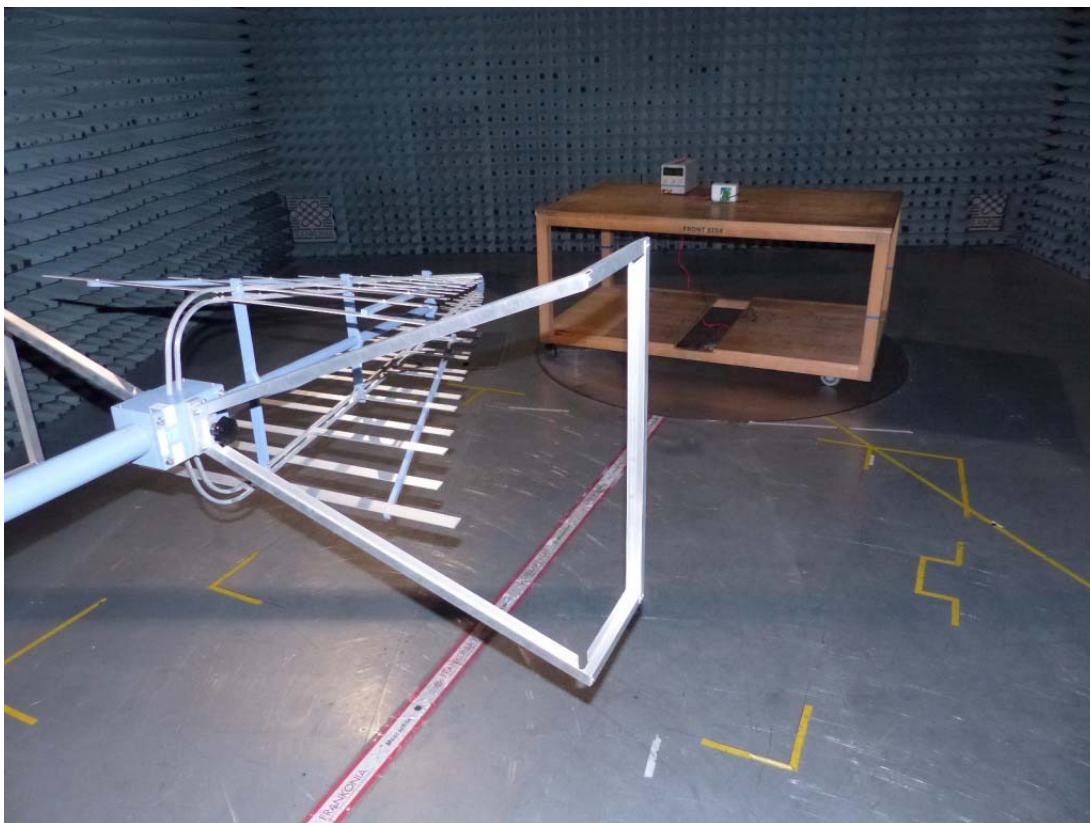
Photo 4: Test setup for radiated measurements (30 MHz to 1 GHz)
