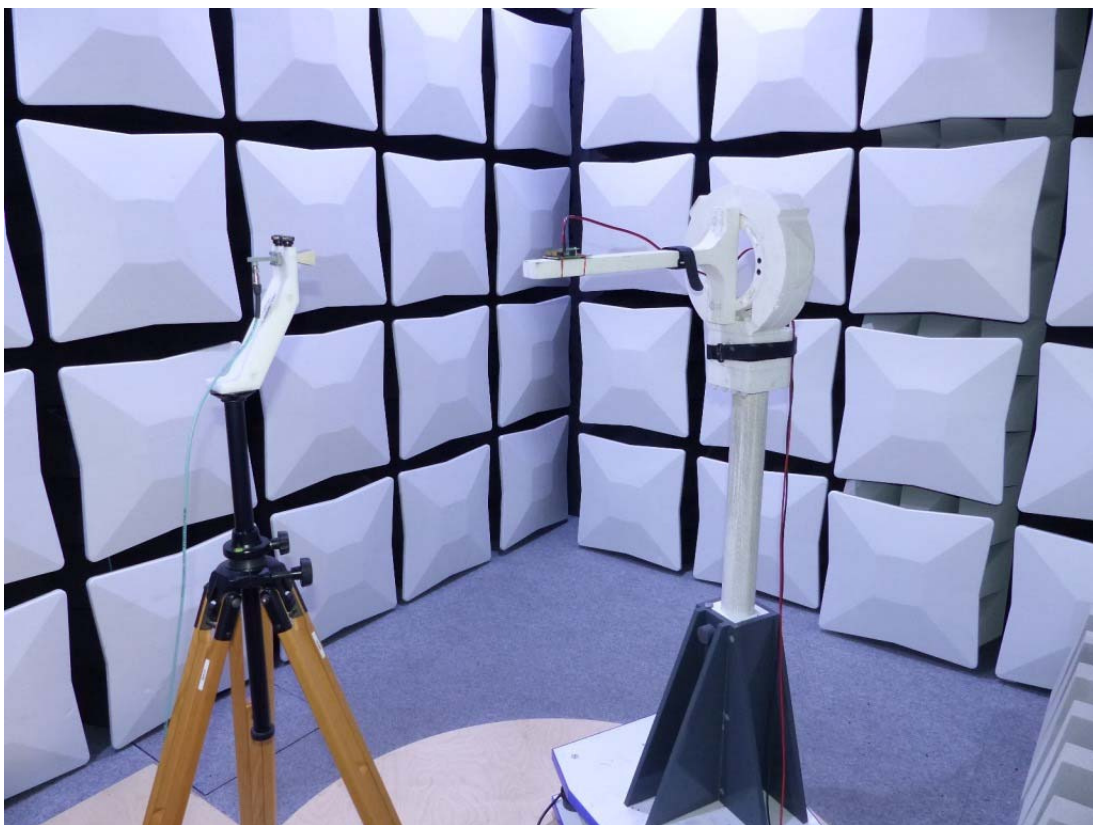
Photo 6: Test setup for radiated measurements above 26 GHz
