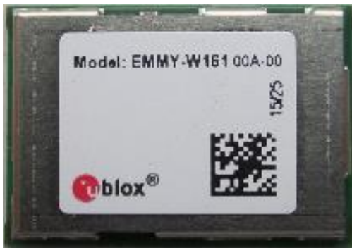
Figure 3: EMMY-W161 top view internal photo
