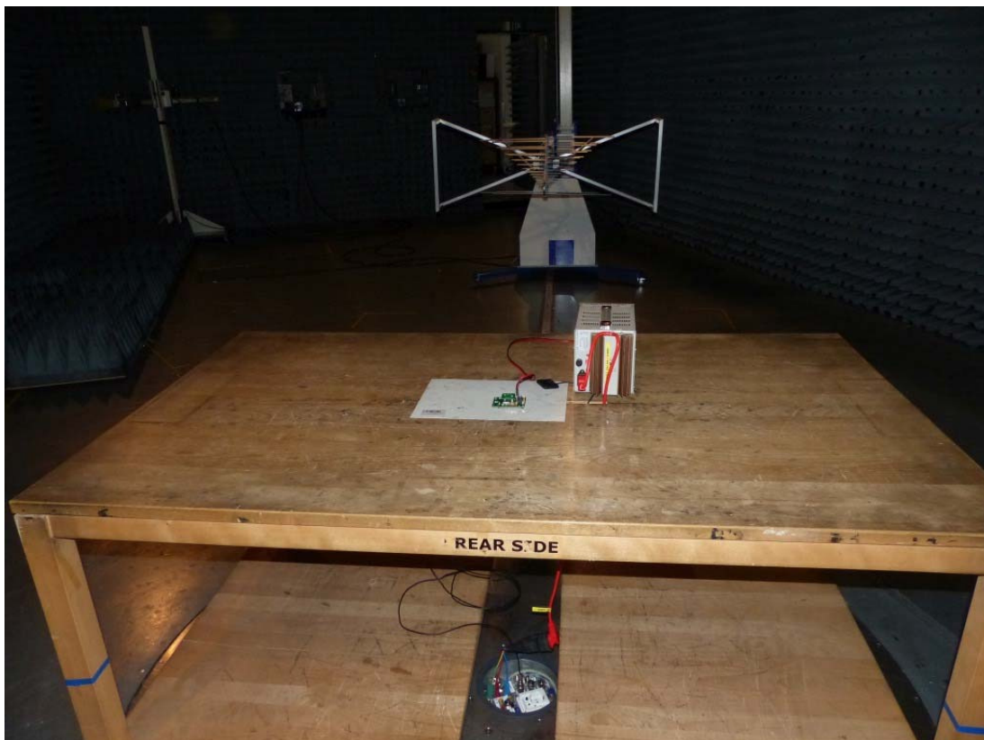
Photo 4: Test setup for radiated measurements below 1 GHz, rear side view)
