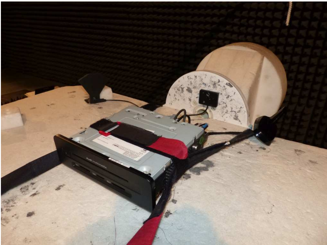
Photo 4: Test setup for radiated measurements (above 1 GHz)
