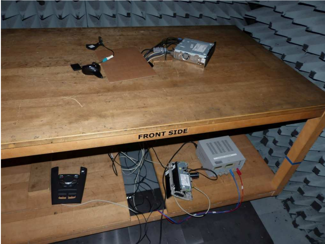
Photo 1: Test setup for radiated measurements (below 30 MHz)
