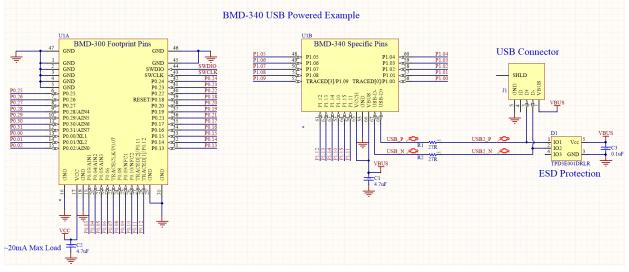
Figure 9: BMD-340/341 USB-powered HV mode example
