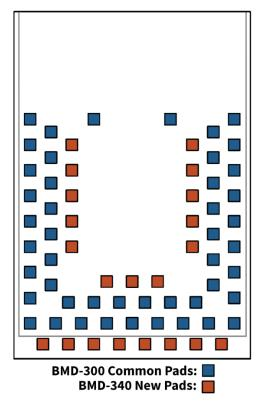
Figure 3: BMD-340/341 and BMD-300/301/330/360 Footprint comparison
