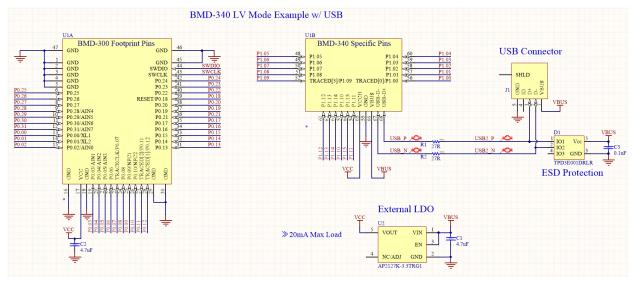
Figure 8: BMD-340/341 LV Mode w/ USB and external regulator
