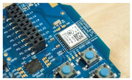
Figure 4: BMD-300 Module soldered to BMD-340/341 footprint
