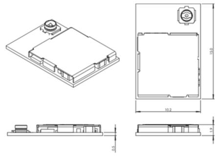
Figure 11: BMD-341 mechanical drawing
