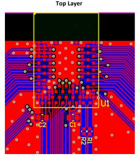
Figure 6: BMD-341 two-layer fan-out example
