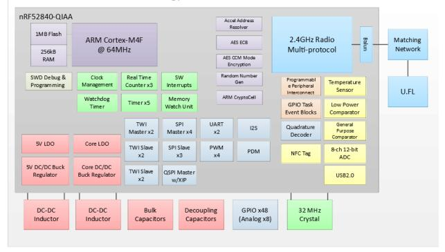
Figure 1: Block diagram of BMD-341
