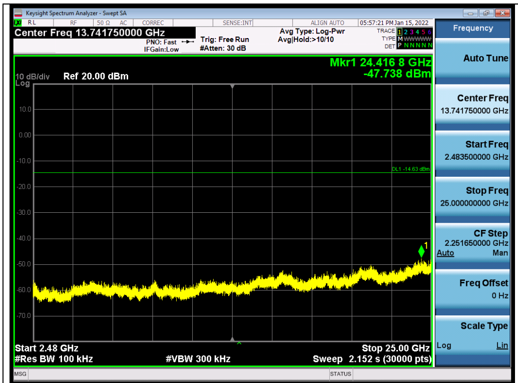
Test_Graph_LE2M_ANT1_2440_2Mbps_Higher Band Emissions
