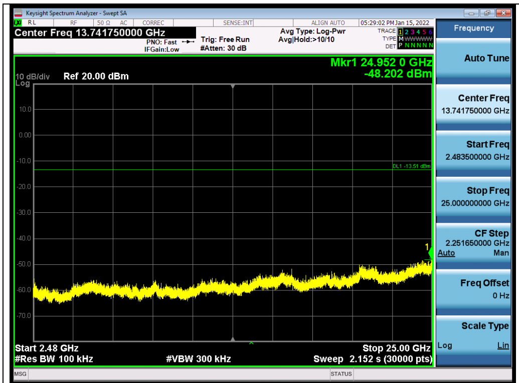
Test_Graph_LE1M_ANT1_2402_1Mbps_Higher Band Emissions
