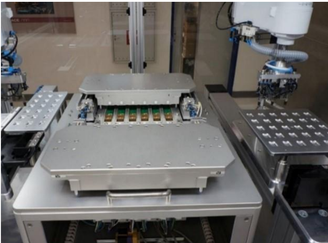
Figure 28: Automatic test equipment for module test
