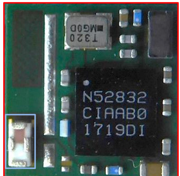
ANNA-B112 module top view with removed cover
