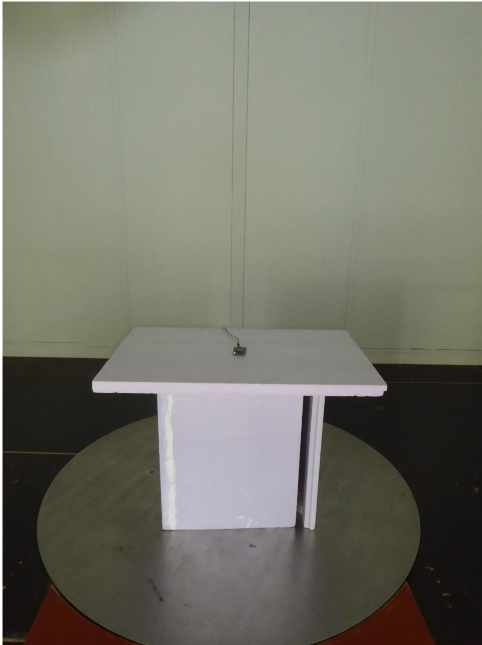
181323_SetRadC8.JPG: Test setup open area test site; EVB-ANNA-B112C#143, 30 MHz – 1 GHz
