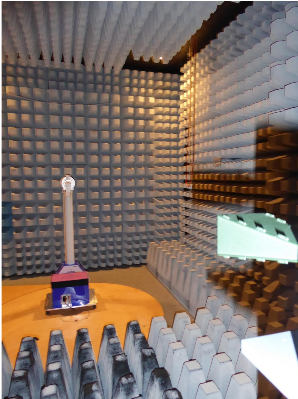
181323_SetRadE11.JPG: Test setup fully anechoic chamber; EVB-ANNA-B112E#143, 18 – 26.5 GHz
