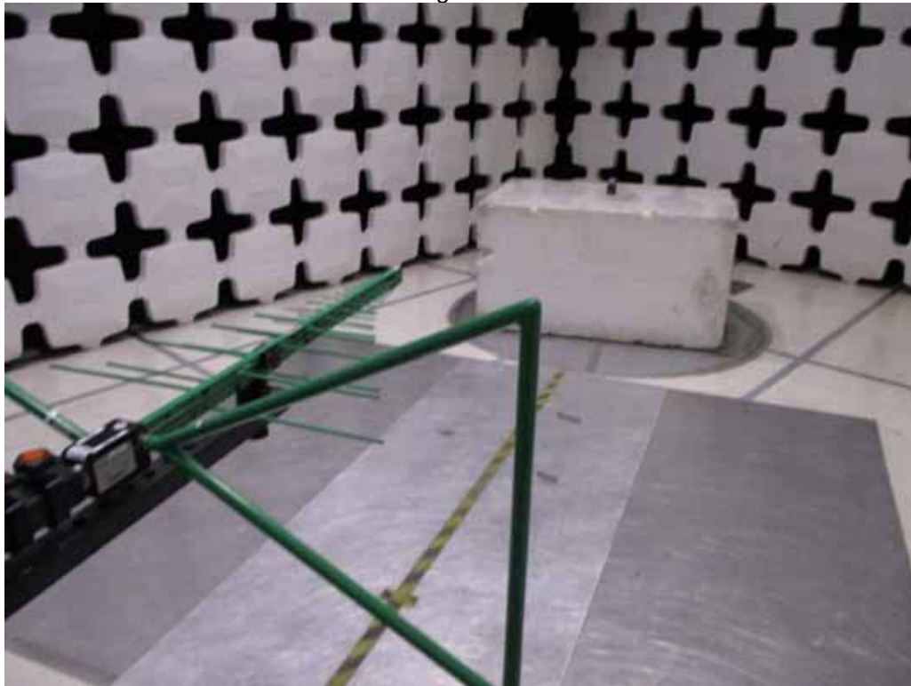
Test Setup for Radiated Emissions – 30MHz to 1000MHz, Horizontal Polarization
