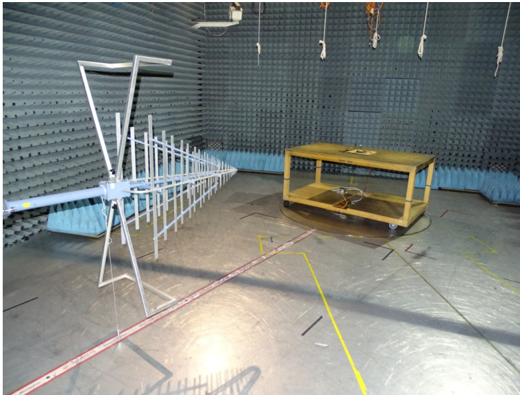
Photo 1: Test setup for radiated measurements
