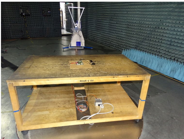
Photo 2: Test setup for radiated measurements
