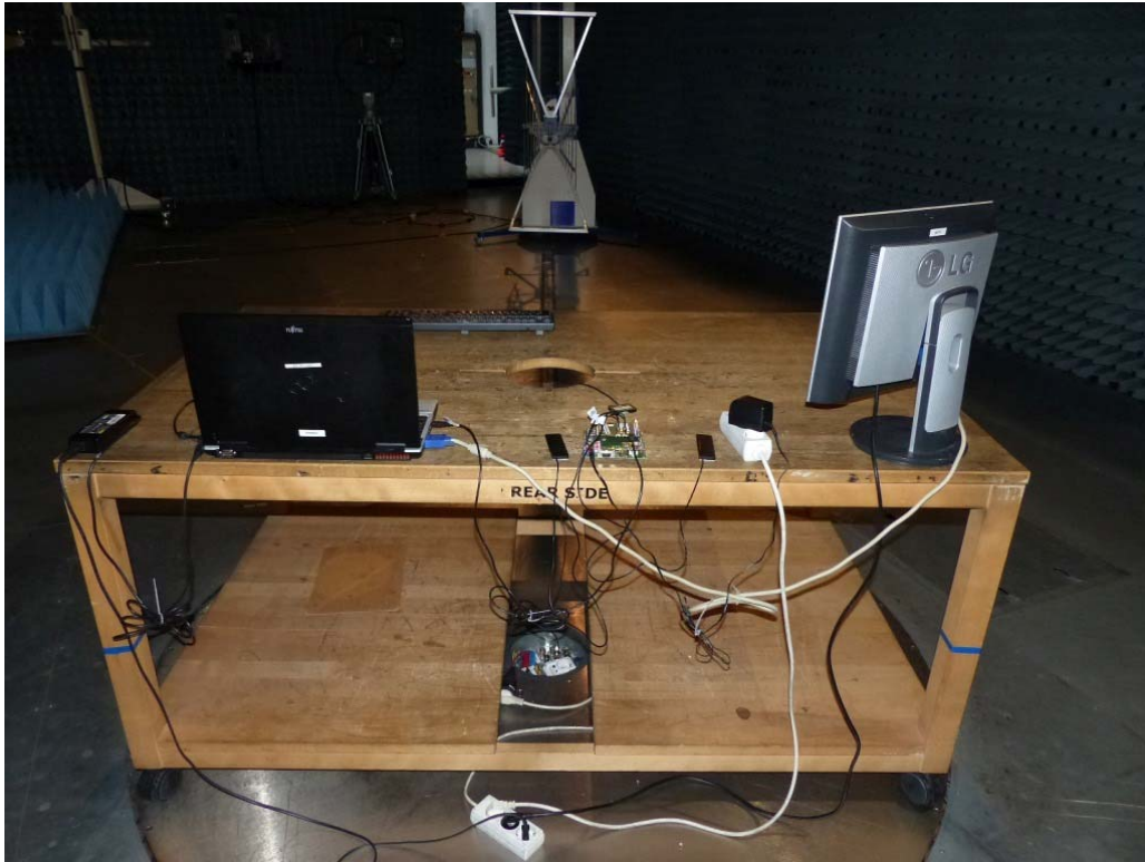
Photo 4: Test setup for radiated measurements (computer peripheral setup, EUT supplied by USB-cable from computer, unintentional radiator $15.109, ANSI C63.4) Below 1 GHz
