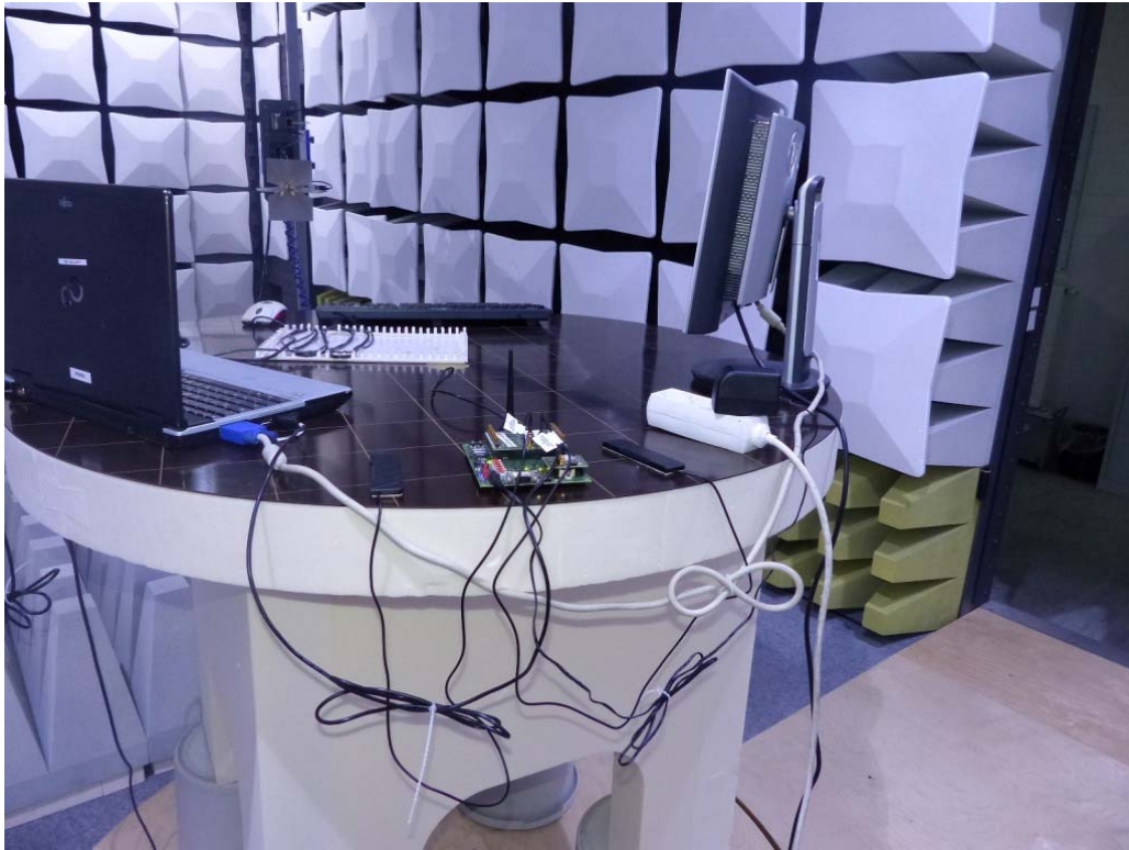
Photo 4: Test setup for radiated measurements (computer peripheral setup, EUT supplied by USB-cable from computer, unintentional radiator §15.109, ANSI C63.4) Above 1GHz
