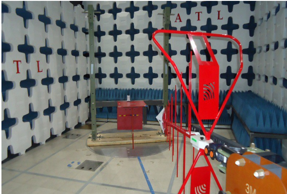
Figure 4.2 - Radiated Emission Test Setup - Front View
