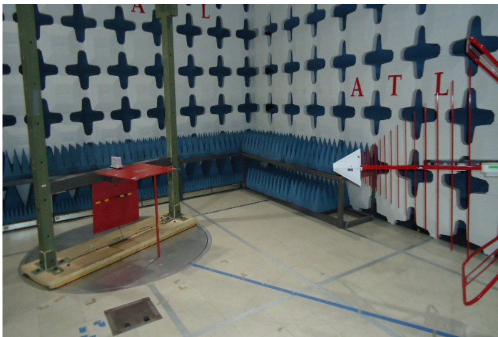
Figure 4.3 - Radiated Emission Test Setup - Side View
