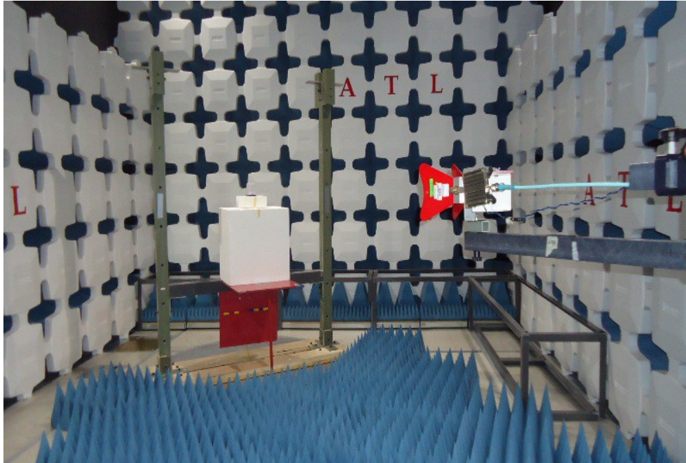
Figure 4.4 - Radiated Emission Test Setup - Front View
