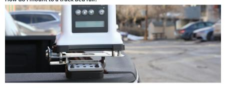
Screw the anchor point into the truck bed rail, and then attach the G7 Bridge Mounting Bracket to the anchor point using screws. Screw the multi-purpose mount to the G7 Bridge Mounting Bracket plate. Slide and snap G7 Bridge into the multi-purpose mount, and lock G7 Bridge Mounting Bracket with key for additional security.
