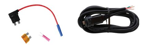
The three-wire hardwire kit and fuse expander can be used to hardwire into a vehicle's 12/24 VDC power system. Plug the fuse expander into a fuse box located on driver's side, and attach the hardwire kit once the fuse expander is in the panel. Ensure cable is properly grounded. Cable routing can be done behind headliner on driver's side and out the rear brake light to the G7 Bridge on the roof, toolbox, or on truck bed rail if it is close to the back windshield.
