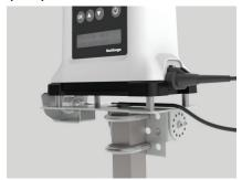
Screw the multi-purpose mount to the G7 Bridge Mounting Bracket plate. Attach the G7 Bridge Mounting Bracket to roof rack, bed rack or pole/post using the appropriate u-bracket size. Slide and snap G7 Bridge into the multi-purpose mount, and lock the G7 Bridge Mounting Bracket with key for additional security.
