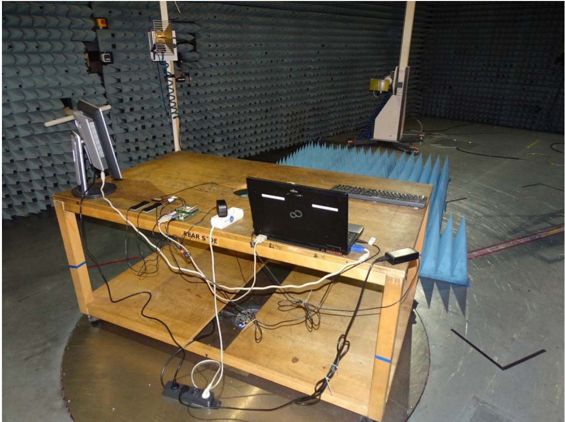
Photo 5: Test setup for radiated measurements (computer peripheral setup, EUT supplied by USB-cable from computer, unintentional radiator §15.109, ANSI C63.4) Above 1GHz
