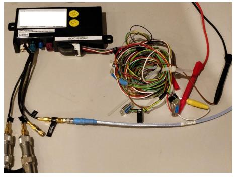
1.2.2. Test Setup for Frequency stability, temperature variation
