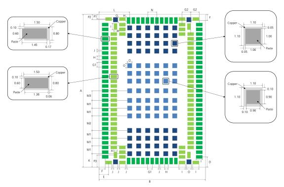
Figure 68: Suggested footprint and stencil design for TOBY-L4 series modules, to be implemented on application PCB (top view)
