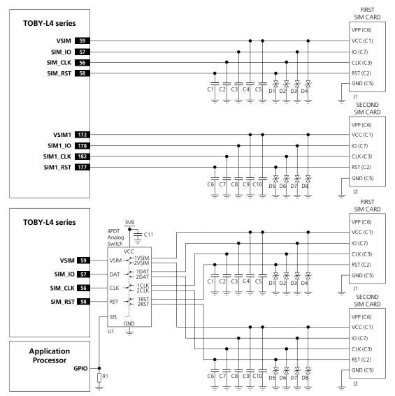
Figure 40: Application circuits for the connection to two removable SIM cards, with SIM detection not implemented
