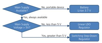
Figure 19: VCC supply concept selection
