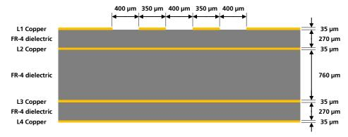
Figure 44: Example of USB line design, with  $Z_0$  close to 90  $\Omega$  and  $Z_{\text{cm}}$  close to 30  $\Omega$ , for the described 4-layer board layup
