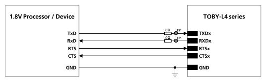
Figure 46: 4-wire UART interface application circuit to connect an external 1.8 V processor / device
