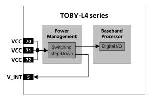
Figure 11: TOBY-L4 series generic digital interfaces supply output (V\_INT) simplified block diagram
