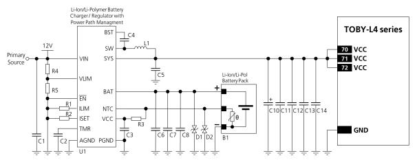
Figure 27: Li-lon (or Li-Polymer) battery charging and power path management application circuit
