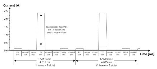
Figure 4: VCC current consumption profile versus time during a 2G single-slot call (1 TX slot, 1 RX slot)
