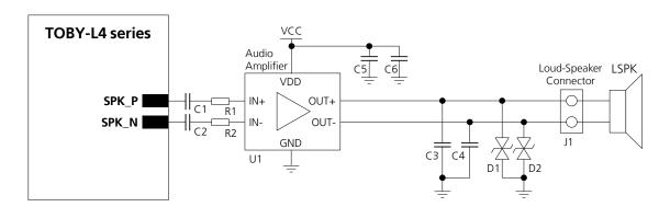
Figure 64: Application circuit connecting the analog audio interface to a high-power loudspeaker
