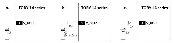
Figure 29: RTC back-up supply (V\_BCKP) application circuits using a capacitor, a super-capacitor, or a non-rechargeable battery
