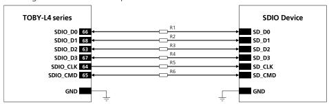
Figure 58: Application circuit for connecting TOBY-L4 series modules to a 1.8 V SDIO device
