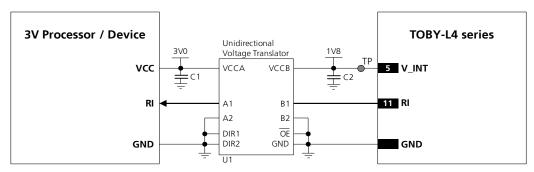
Figure 51: Ring Indicator application circuit to connect an external 3.0V processor / device
