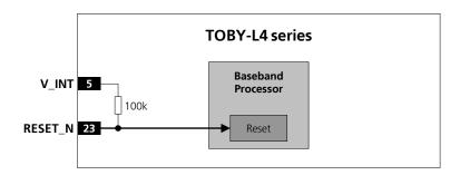
Figure 15: TOBY-L4 series RESET\_N input equivalent circuit description
