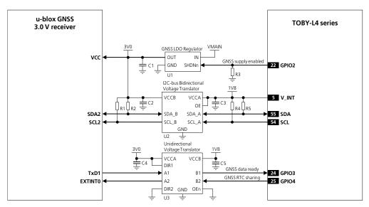
Figure 56: Application circuit for connecting TOBY-L4 series modules to u-blox 3.0 V GNSS receivers
