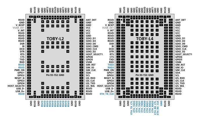
Figure 72: TOBY-L2 and TOBY-L4 series modules pad layout and pin assignment
