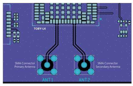
Figure 35: Example of the circuit and layout for antenna RF circuits on the application board
