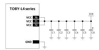
Figure 24: Suggested schematic for the VCC bypass capacitors to reduce ripple / noise on the supply voltage profile
