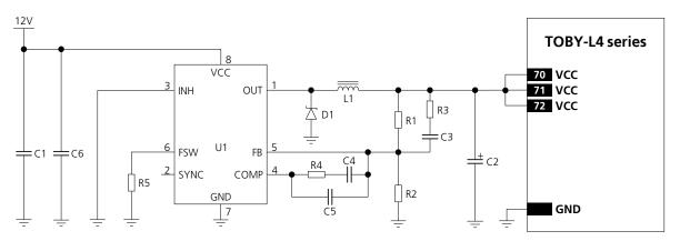
Figure 21: Example of low cost VCC supply application circuit using a step-down regulator
