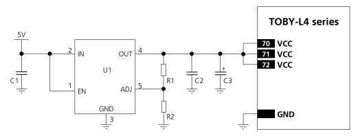
Figure 23: Example of a low cost VCC supply application circuit using an LDO linear regulator
