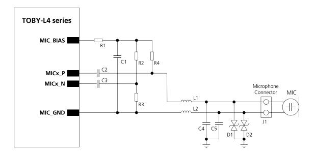
Figure 61: Application circuit connecting the analog audio interface to one external electret microphone
