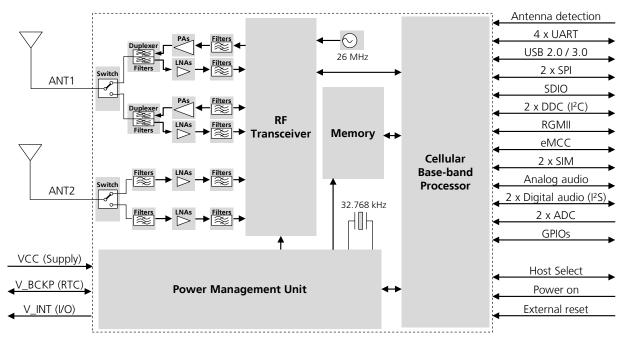
Figure 1: TOBY-L4 series modules simplified block diagram
