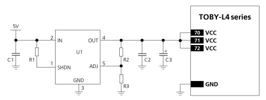
Figure 22: Example of high reliability VCC supply application circuit using an LDO linear regulator
