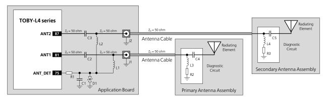
Figure 36: Suggested schematic for the antenna detection circuit on the application board and the diagnostic circuit on the antennas assembly
