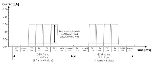
Figure 6: VCC current consumption profile during a 2G GPRS/EDGE multi-slot connection (4 TX slots, 1 RX slot)
