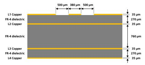
Figure 33: Example of a 50  $\Omega$  coplanar waveguide transmission line design for the described 4-layer board layup
