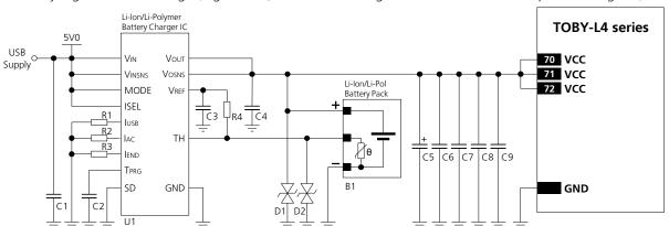
Figure 25: Li-lon (or Li-Polymer) battery charging application circuit
