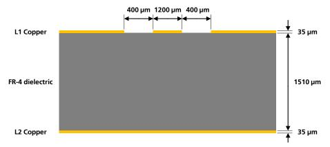
Figure 34: Example of a 50  $\Omega$  coplanar waveguide transmission line design for the described 2-layer board layup
