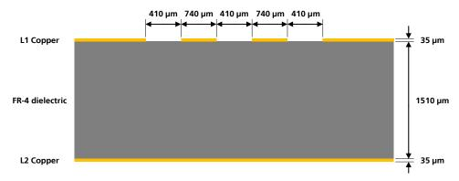
Figure 45: Example of USB line design, with  $Z_0$  close to 90  $\Omega$  and  $Z_{CM}$  close to 30  $\Omega$ , for the described 2-layer board layup
