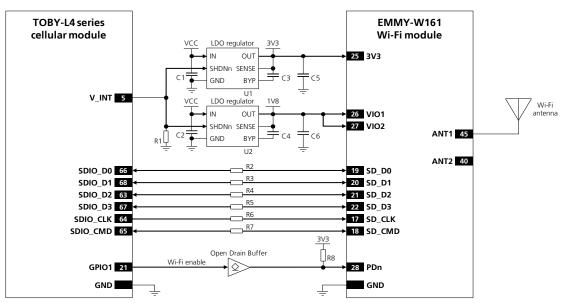
Figure 57: Application circuit for TOBY-L4 cellular module and u-blox EMMY-W161 short range radio communication module
