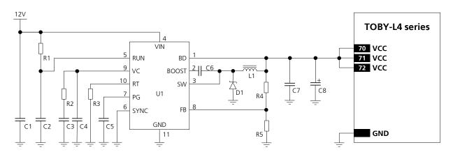
Figure 20: Example of high reliability VCC supply application circuit using a step-down regulator
