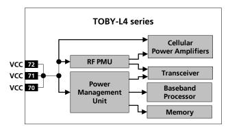
Figure 3: TOBY-L4 series modules' internal VCC supply routing simplified block diagram
