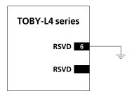
Figure 67: Application circuit for the reserved pins (RSVD)
