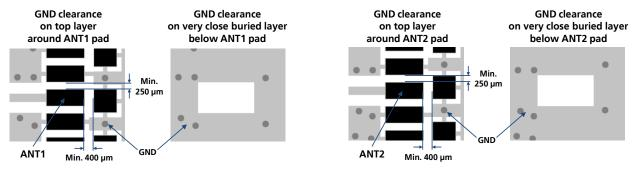
Figure 32: GND keep-out area on top layer around ANT1 / ANT2 pads and on very close buried layer below ANT1 / ANT2 pads
