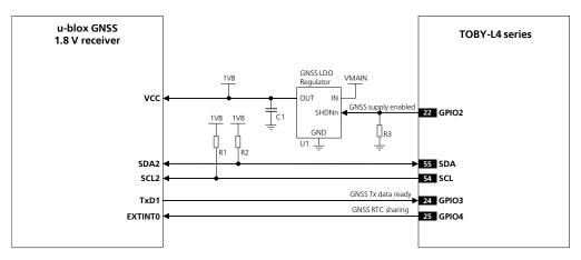
Figure 54: Application circuit for connecting TOBY-L4 series modules to u-blox 1.8 V GNSS receivers
