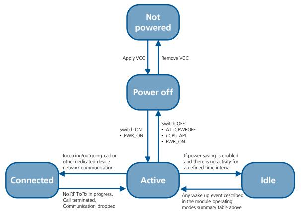
Figure 2: TOBY-L4 series modules operating modes transitions
