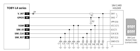
Figure 39: Application circuit for the connection to a single removable SIM card, with SIM detection implemented
