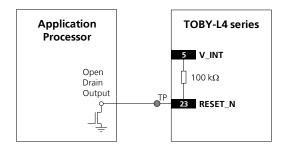
Figure 31: RESET\_N application circuits using a push button and an open drain output of an application processor
