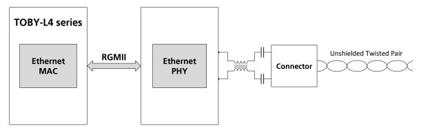
Figure 59: RGMII interface application circuit block diagram
