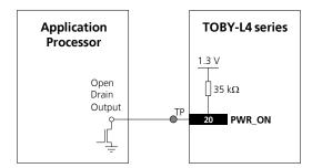
Figure 30: PWR\_ON application circuits using a push button and an open drain output of an application processor
