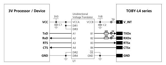
Figure 47: 4-wire UART interface application circuit to connect an external 3.0V processor / device
