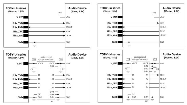
Figure 66: I'S interface application circuit with an external audio codec to provide voice capability
