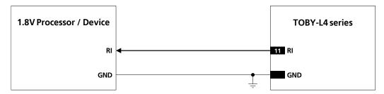
Figure 50: Ring Indicator application circuit to connect an external 1.8V processor / device
