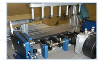
Figure 70: Automatic test equipment for module tests
