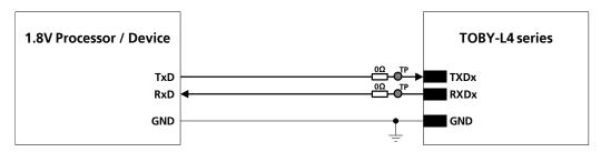
Figure 48: 2-wire UART interface application circuit to connect an external 1.8V processor / device
