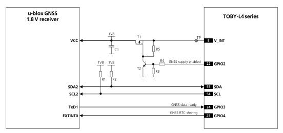
Figure 55: Application circuit for connecting TOBY-L4 series modules to u-blox 1.8 V GNSS receivers using V\_INT as supply
