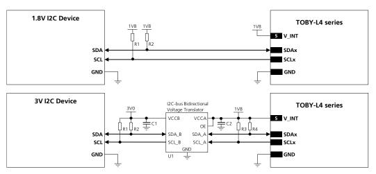
Figure 53: Application circuit for connecting TOBY-L4 series modules to 1.8 V or 3 V I2C devices
