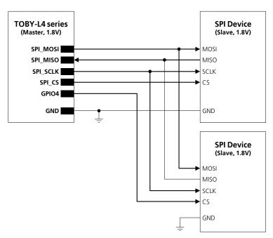
Figure 52: SPI interface application circuit for connecting two external SPI slave devices
