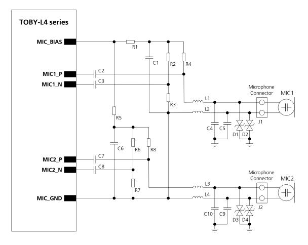
Figure 60: Application circuit connecting the analog audio interface to two external electret microphones
