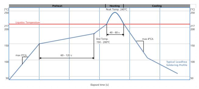
Figure 69: Recommended soldering profile
