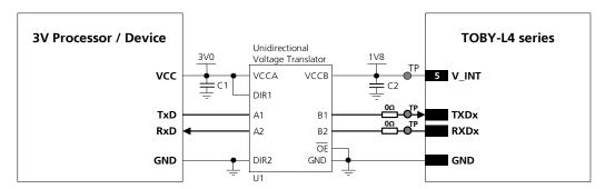
Figure 49: 2-wire UART interface application circuit to connect an external 3.0 V processor / device
