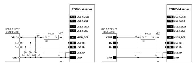
Figure 42: USB 2.0 interface application circuits, with TOBY-L4 series module acting as a USB host
