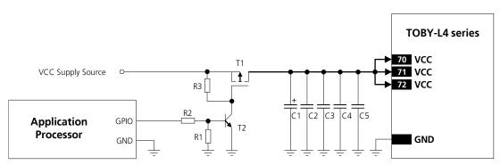
Figure 28: Example of application circuit for VCC supply removal
