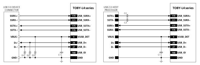
Figure 43: USB 3.0 interface application circuits, with TOBY-L4 series module acting as a USB device
