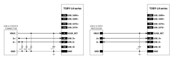
Figure 41: USB 2.0 interface application circuits, with TOBY-L4 series module acting as a USB device
