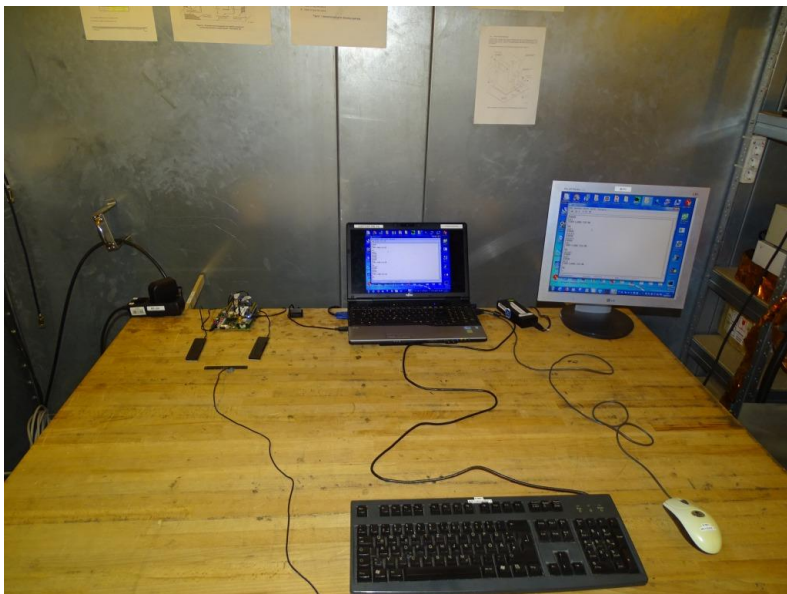
Photo 1: Test setup for conducted measurements
