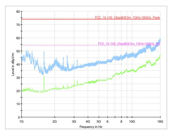
AC mains connection = via ANC1, Measurement range = 1 GHz - 18 GHz, Test setup = computer peripheric (S01\_BA01)
