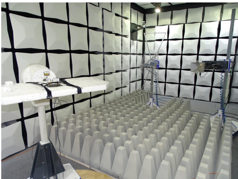
Photo 2: Test setup for radiated measurements (below 1 GHz)
