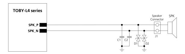
Figure 63: Application circuit connecting the analog audio interface to a low-power speaker
