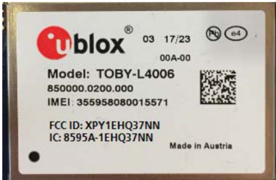
Top with shielding installed.
