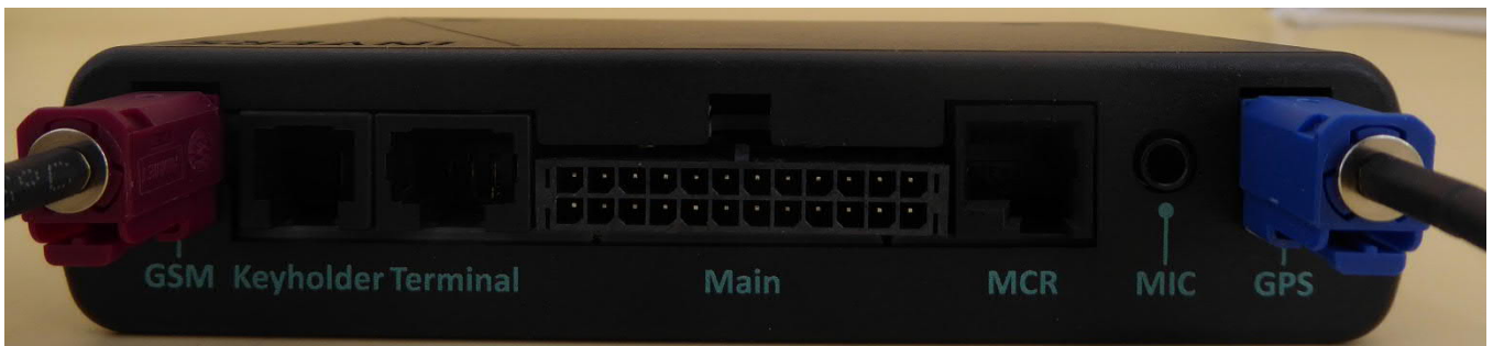
Rear Ports and antenna connectors
