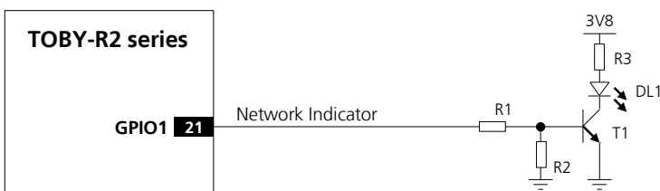
Figure 65: Application circuit for network indication provided over GPIO1
