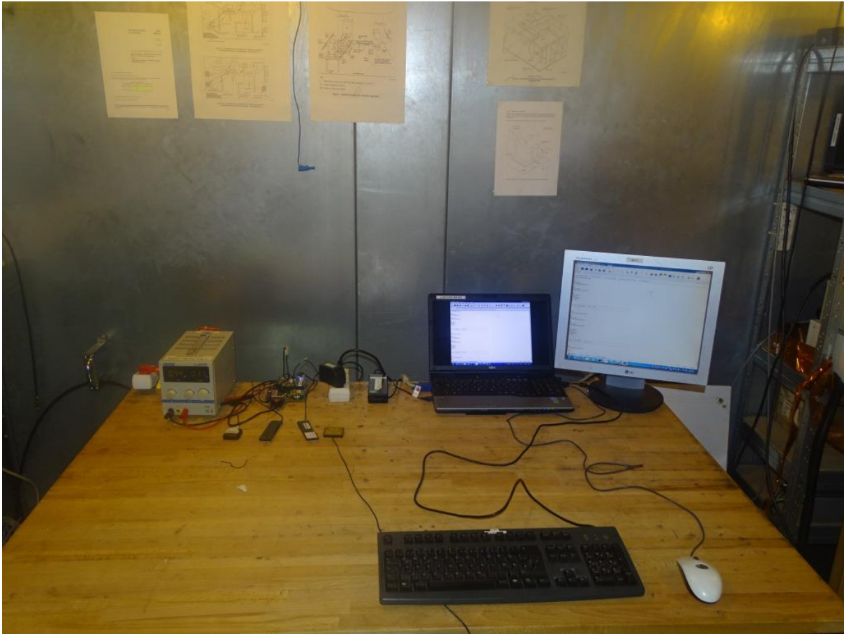
Photo 3: Test setup for conducted measurements (computer peripheral setup, EUT supplied by USB-cable from computer, unintentional radiator §15.107, ANSI C63.4)
