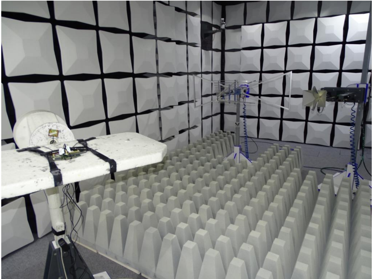
Photo 1: Test setup for radiated measurements (Enclosure, fully-anechoic chamber, 1-18 GHz intentional radiator §15 / 30 MHz – 10/20 GHz §22/24/27)
