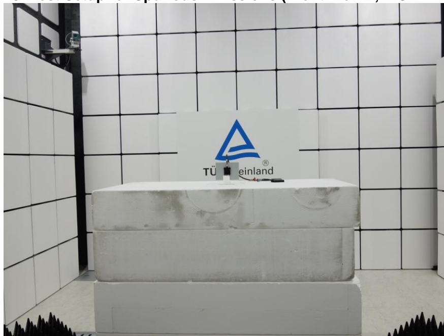
Photograph 18: Test Setup for Spurious Emissions (Front View 2, WCDMA Band II)
