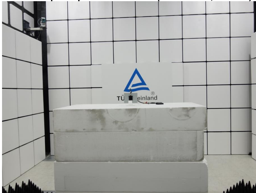
Photograph 6: Test Setup for Spurious Emissions (Front View 2, WCDMA)
