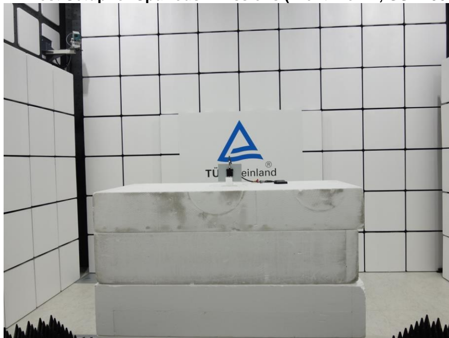
Photograph 14: Test Setup for Spurious Emissions (Front View 2, GSM1900)
