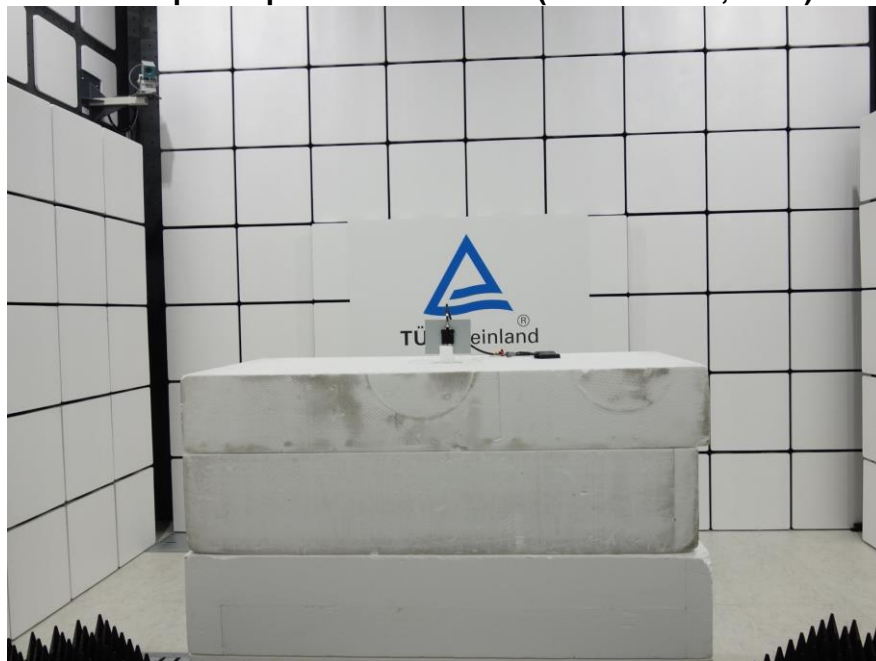
Photograph 2: Test Setup for Spurious Emissions (Front View 2, GSM)
