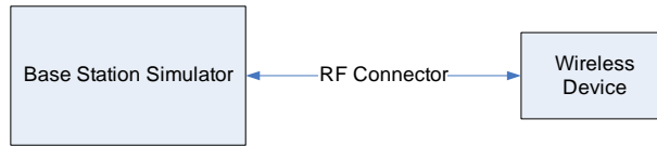
Figure 7-1 Power Measurement Setup
