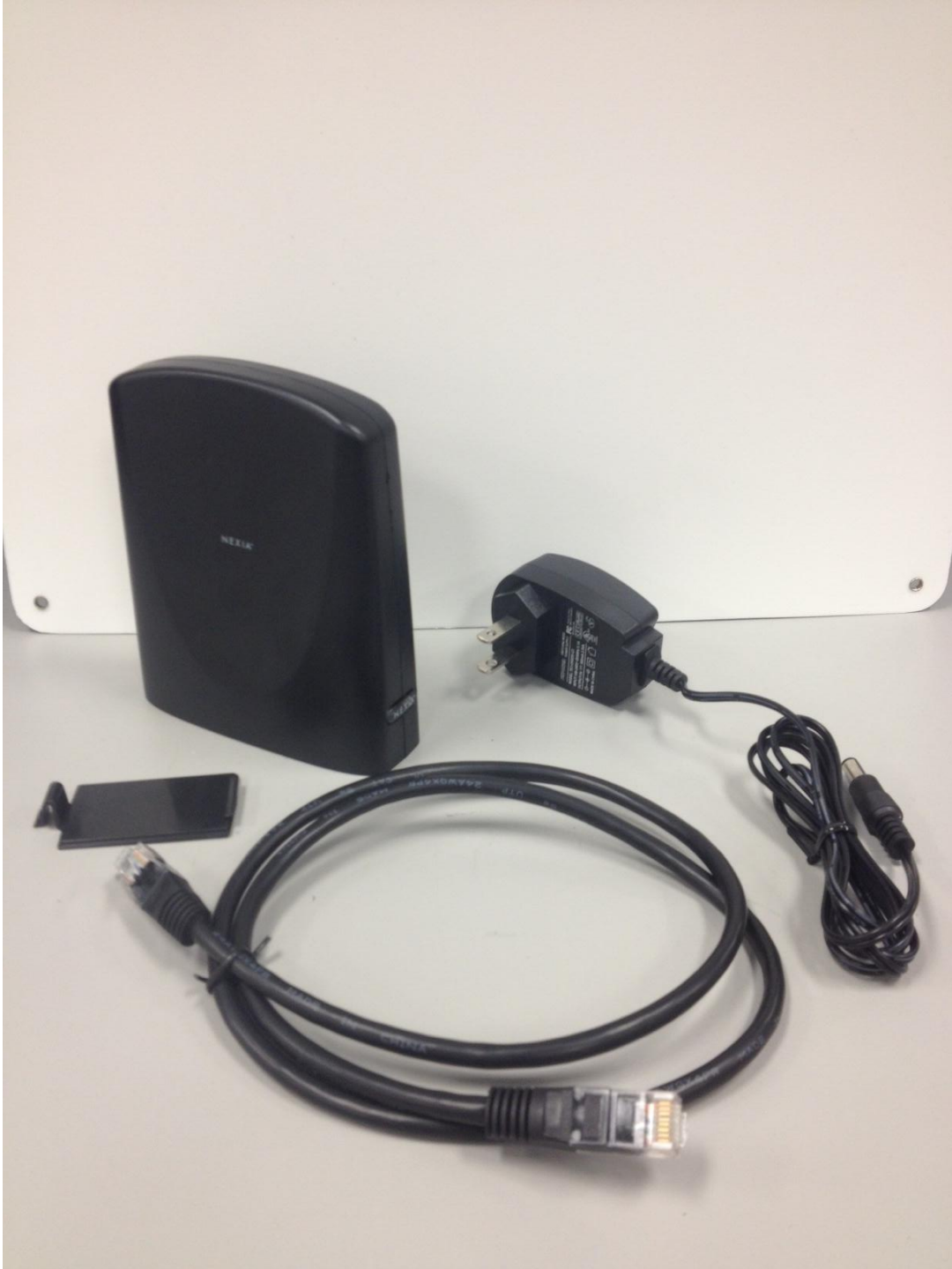
IMAGE 1: Gen2 Bridge (Equipment under test) with all outside connection equipment. Included: Ethernet cable, 5V power supply, and battery cover.
