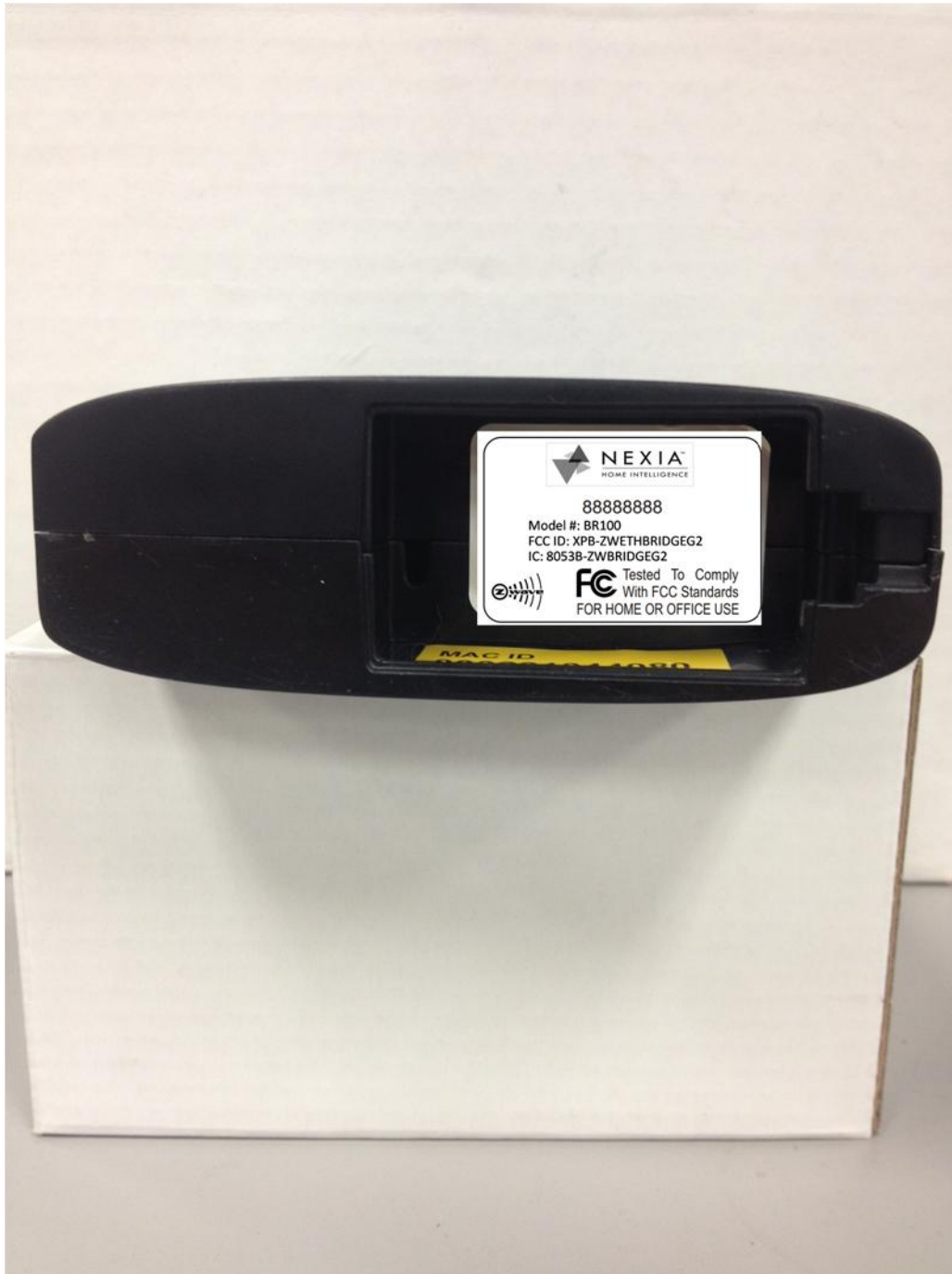
IMAGE 2: View from underside of EUT displaying FCC label information including FCC ID. Mock-up of decal displayed. Battery cover not shown.
