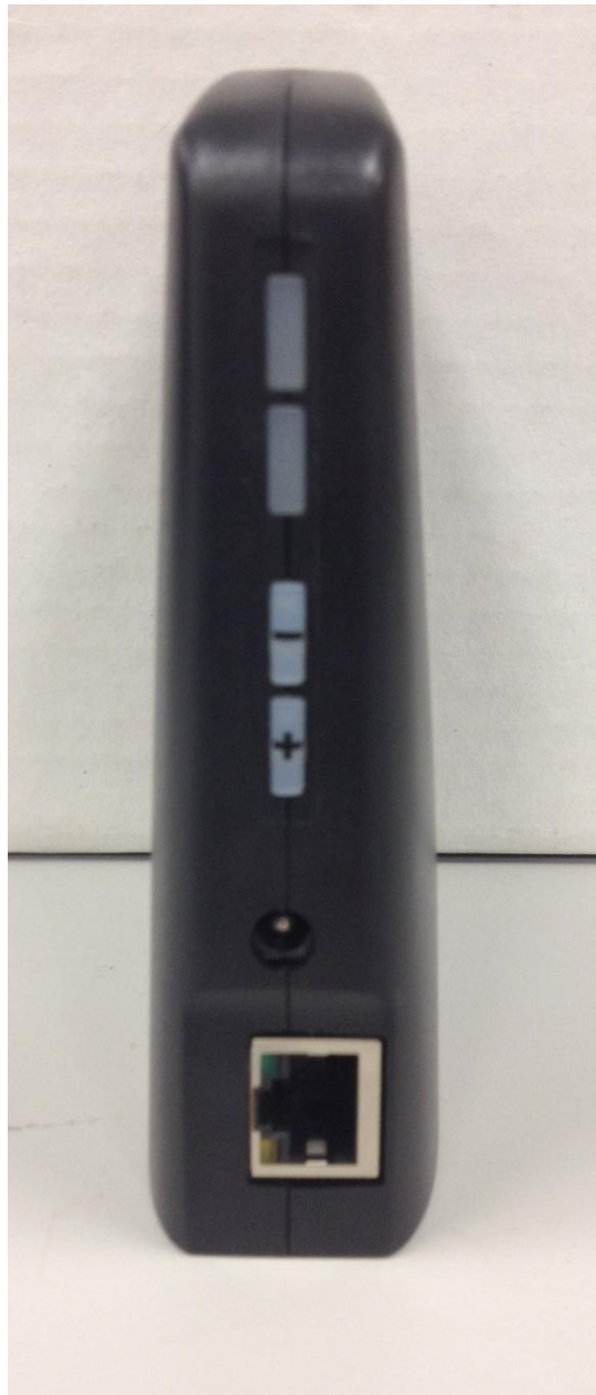
Image 6: Rear of EUT displaying silicone light display points at top, two buttons with negative and positive labels, 5V power supply input point, Ethernet Connection point.
