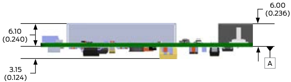
Figure 1.3: Vertical height of tallest component off of the OEM 200 Main board mm (inches).
