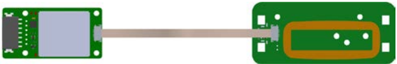
Figure 1.1: OEM 200 main board connected to an 80mm antenna board via 4 inch flexible cable (Top View)
