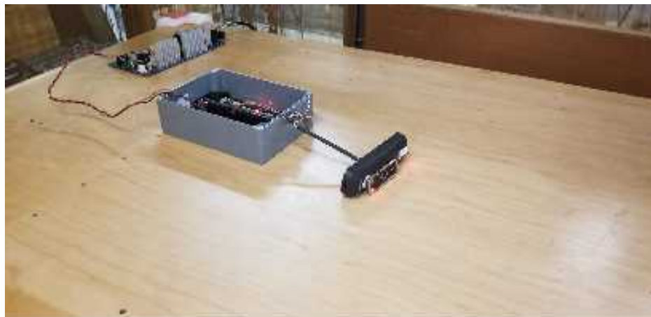
Figure 6: Conducted Emissions Test Setup Photograph(s).
