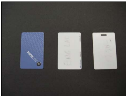
From left to right: Setup ID card for setting different transmit modes, 13.56MHz ID card and 125kHz ID card. These cards were used to set EUT in test mode and test for functionality of the PROX reader.
