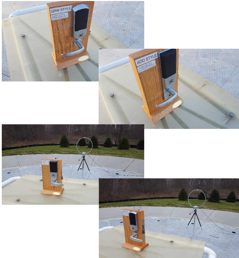
Figure 4: Radiated Emissions Test Setup Photograph(s).
