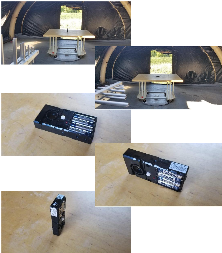
Figure 4: Radiated Emissions Test Setup Photograph(s).
