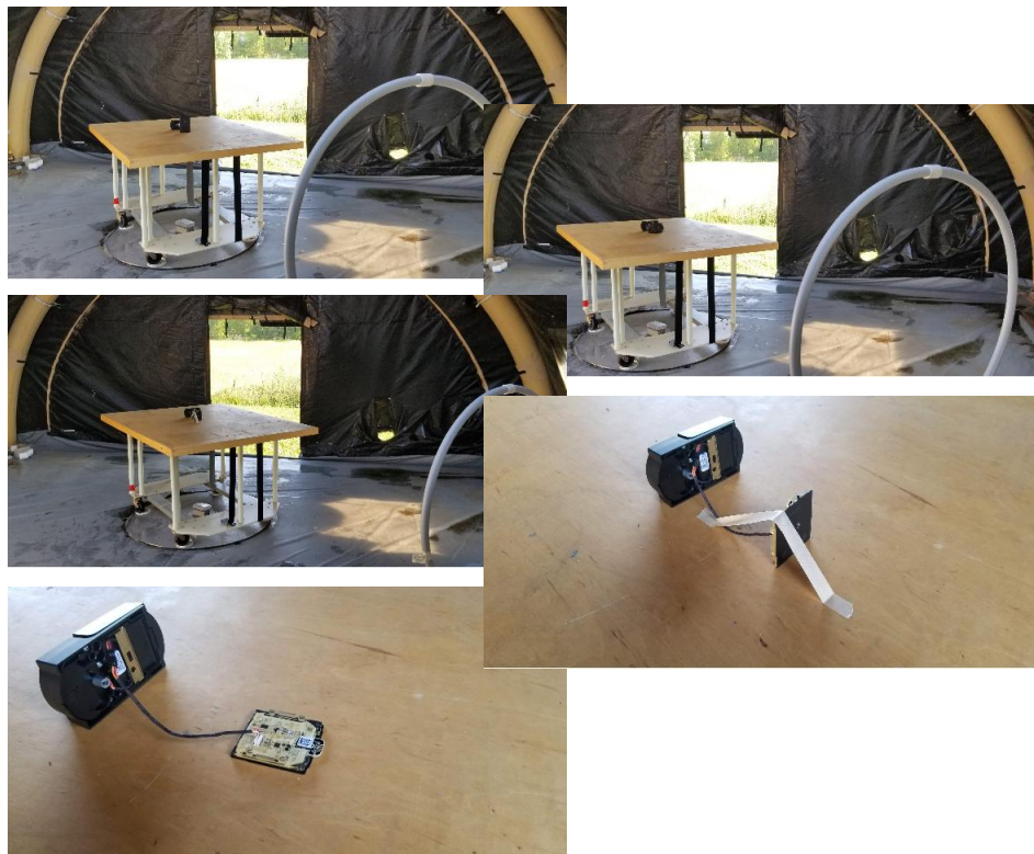
Figure 4: Radiated Emissions Test Setup Photograph(s).
